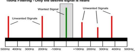
100Hz Filtering - Only the desired signal is heard
