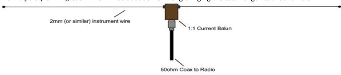
A dipole usually offers a high take-off angle unless it can be raised to a 1/4wave above ground. Dipoles are usually installed flat-top, so that they are the same height at each end and in the middle.
